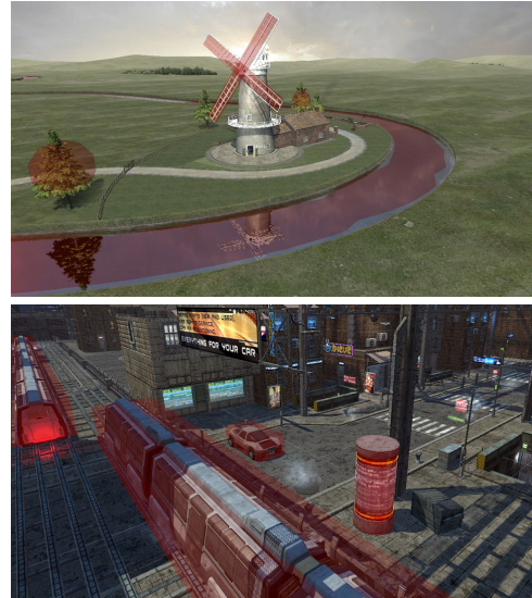
Fig. 4: This visualization shows the sound sources for the windmill and city scenes in red. In the windmill scene, box sound shapes are used to represent the windmill sails, spheres are used for trees, and a triangle mesh is used for the nearby river. In the city, the train and car sound sources are represented by boxes, while scrolling advertisements are represented using meshes that correspond to the visual geometry.
